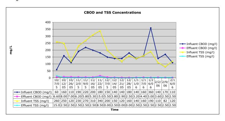
It is important to note the difference between the influent and effluent CBOD, which is a measure of the strength of the wastewater. The influent test BOD is very typical of that from the septic tank in a residential dwelling.
